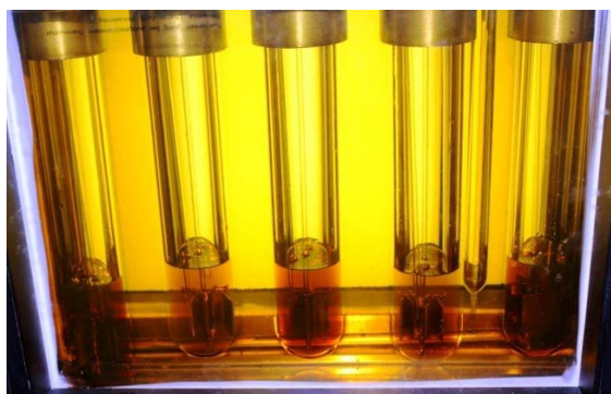
Slika 1. Aparatura za metodu ASTM D 6594 Figure 1. Apparatus for the method ASTM D 6594
