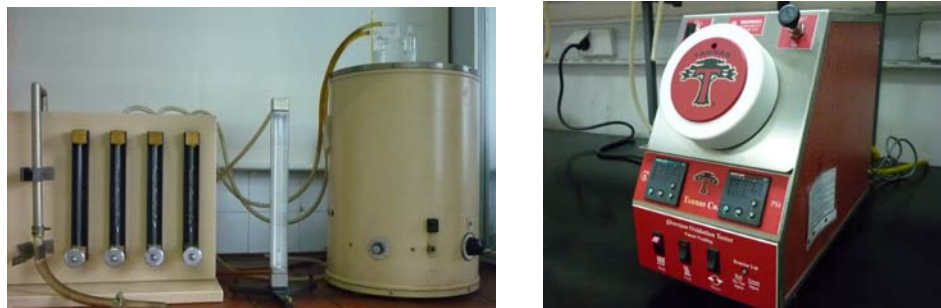
Slika 1. Aparatura za metodu IP 48 i ASTM D2272 Picture 1. Aparature for methods IP 48 and ASTM D2272
